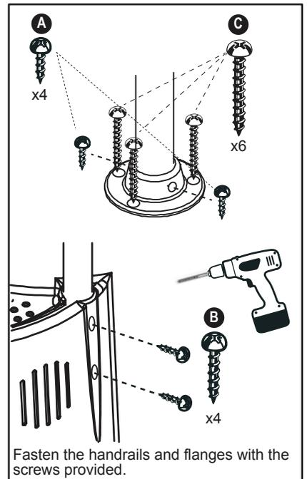
Fasten the handrails and flanges with the screws provided.
