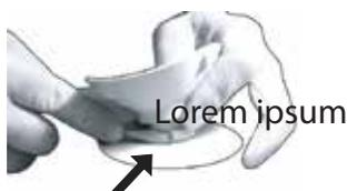
2) With a flat screwdriver, compress the Step Cup™ mushroom ring while pushing it into the hole.
