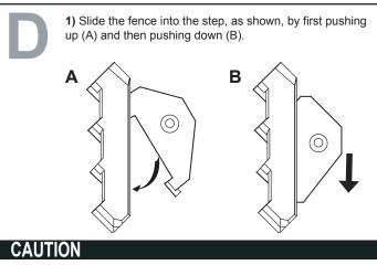
The safety fence should never touch either the bottom or the pool wall.
