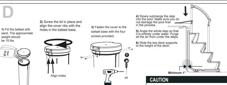
To prevent pool liner puncture, keep a minimum 1" gap between the pool liner and the rear underside of the step.
