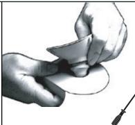
C1) Insert half of the Step Cup mushroom ring in the hole, at a 45 degree angle.
