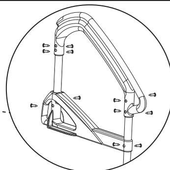
1) Secure the lateral supports and the handrails to the posts using the screws provided.
