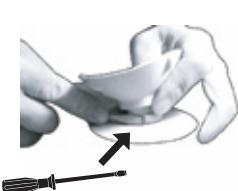
**A2**) With a flat screwdriver, compress the Step Cup mushroom ring while pushing it into the hole.
