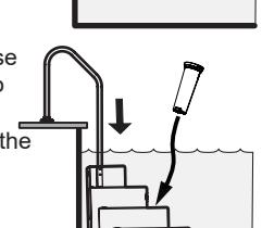
6) Keep a gap of 1" between the step and the pool wall.
