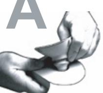
**A1**) Insert half of the Step Cup mushroom ring in the hole, at a 45 degree angle.
