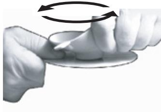
**A3)** Twist the Step Cup to ensure that the mushroom ring has entirely cleared the wall thickness. If it has, the suction cup should rotate freely.
